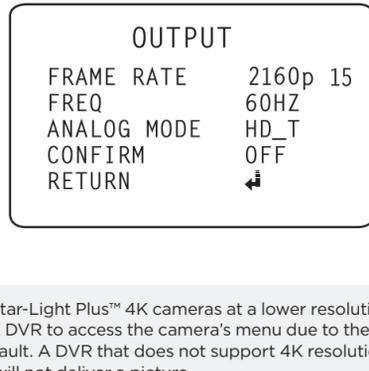
**NOTE:** To use your Star-Light Plus™ 4K cameras at a lower resolution, you must use a VMAX® A1 4K DVR to access the camera's menu due to the cameras being set to 4K as the default. A DVR that does not support 4K resolution may recognize the camera, but will not deliver a picture.
